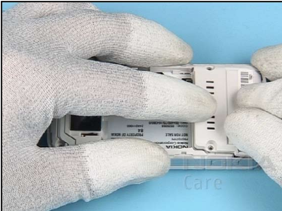
21. Click the snaps of the MAIN ANTENNA COVER ASSEMBLY into their place. Check the correct position before going on.
