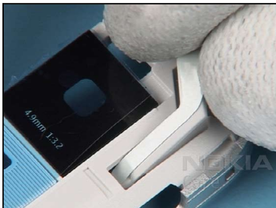
2. Insert the BT ASSEMBLY.
