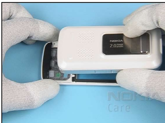
15. Insert the assembly into the A-COVER, beginning from the bottom.
