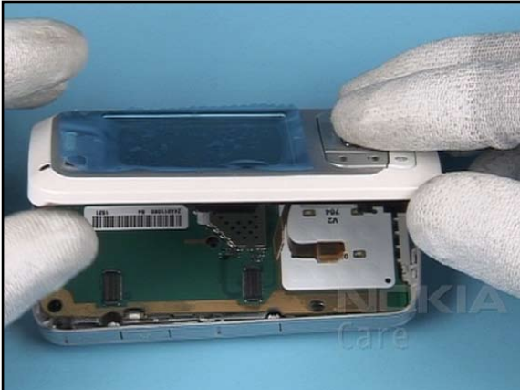
15. Now the parts can be separated.
