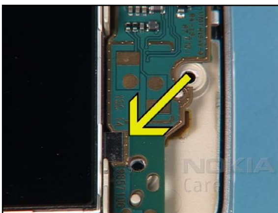
6. Mind the correct positioning of the grounding pad.
