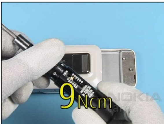
18. Set the correct torque.
