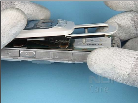
13. Note that both parts are still connected with the flex foils.
