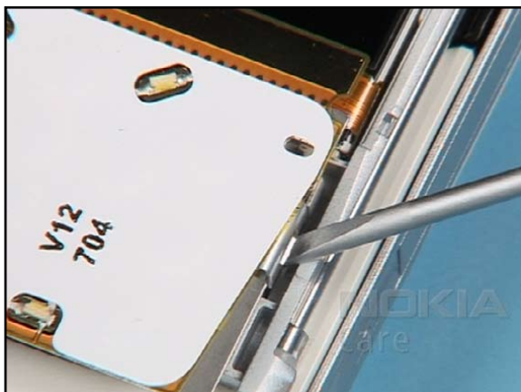
15. Open the metal latches of the SHIELD...
