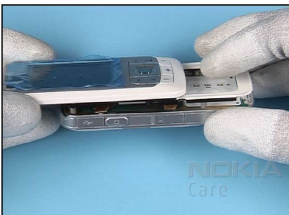
17. Open the slider. Position the upper part over the lower part.
