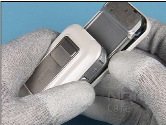
9. Open the clips of the A-COVER.
