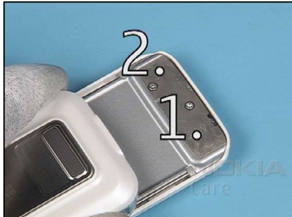
8. Unscrew both screws. It is not necessary the 2nd screw if only A-COVER or FUNCTIONAL KEYMAT needs to be replaced.
