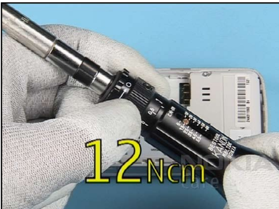
23. Set the correct torque.
