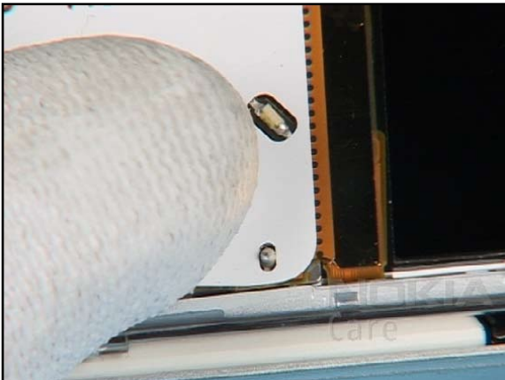
9. Click the snaps into their places. Note the correct positioning of the alignment tabs.
