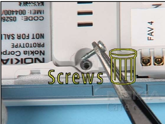
9. Due to the fact that these screws are using locking compound, they must always be replaced after unscrewing.
