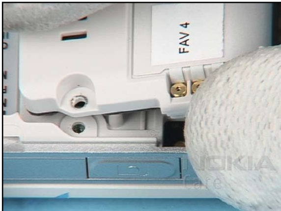
10. Lift up the MAIN ANTENNA COVER ASSEMBLY.
