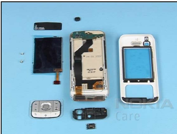
21. The disassembly procedure is now completed.
