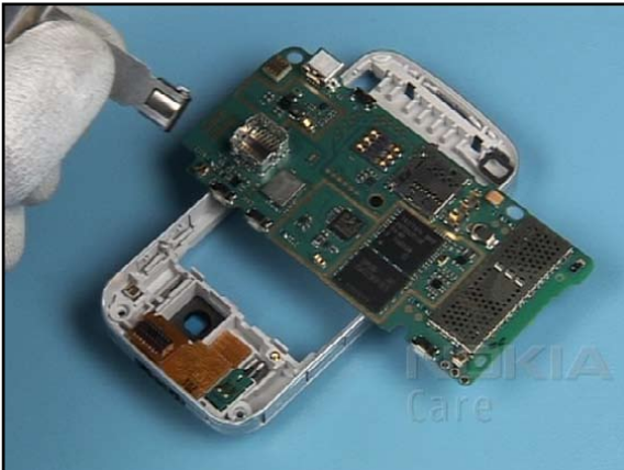
7. Insert the CAMERA MODULE.
