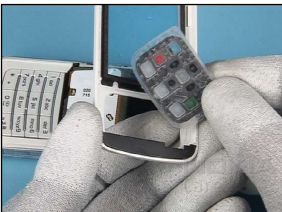
11. The FUNCTIONAL KEYMAT can be removed easily.
