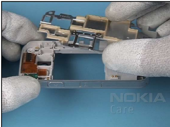
10. Insert the SHIELD LID into the B-COVER.
