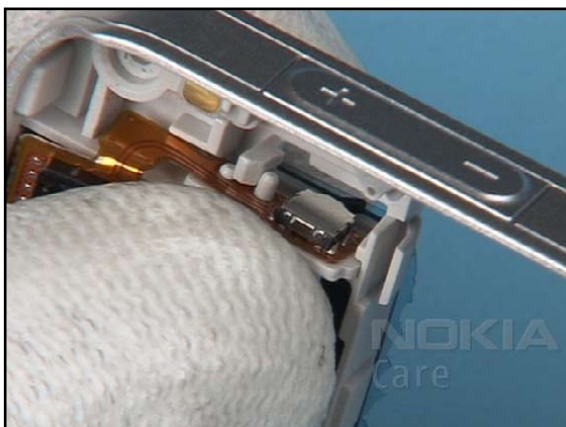
4. Position the switch as shown.
