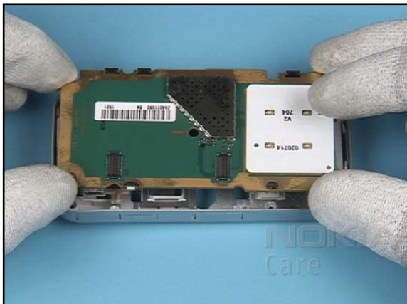
12. Place the ENGINE MODULE.
