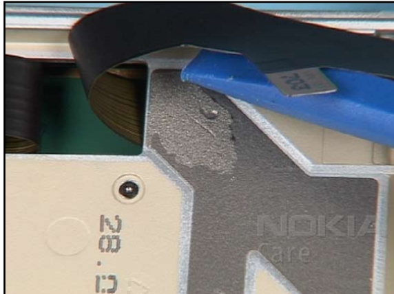
20. The glued in UI FLEX can be removed. Note: For disconnecting the flex connectors the lower block must be disassembled first. The adhesive was assembled for production issues and must not be replaced.
