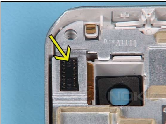
11. Note the correct positioning of the spring contacts as shown before continue.
